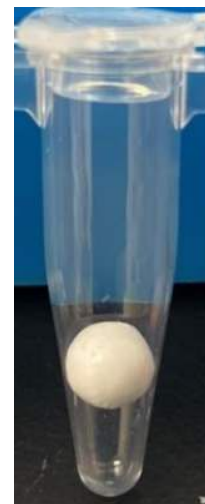
Figure 1. LyoDose bead, a sphere of lyophilized reagents that can be used to support a single reaction in a device or well, shown in a tube. These applications of LyoDose beads have been successful for years. The incorporation of lyophilized
