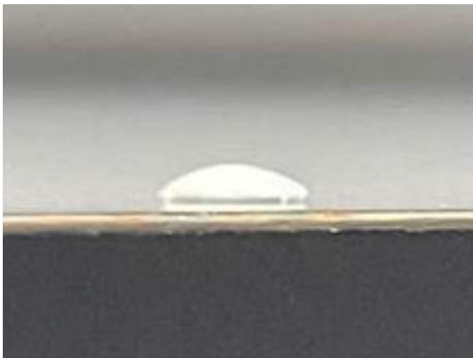
Figure 2. Top view image of LyoDots (A) with a diameter of 3.75 mm. Side view image of a LyoDot (B) with a thickness of 390 \mu\text{m} . The LyoDots consisted of reagents needed for the CDC 2019-nCoV RT-PCR assay, which were provided by Fortis Life Sciences.
